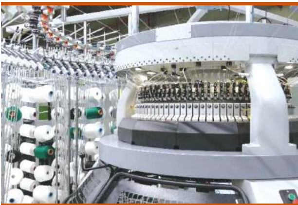
The OVJA 2.4 EC II is equipped with a new system for electronic single needle selection; one of the advantages is a significantly lower knitting head.
