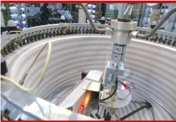
knithawk is a tool for optical defect detection. He sits directly at the knitting point
